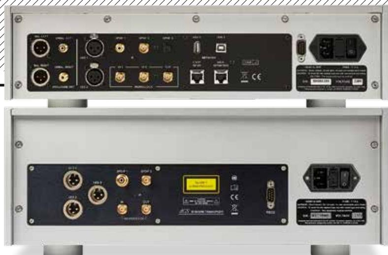
**ABOVE:** Transport [bottom] offers CD and downsampled SACD digital out on S/PDIF (coax and BNC) and AES (XLR). Upsampled DXD and native SACD is output on dual-AES connections. Clock in/outs are mirrored on DAC [top] with three S/PDIF ins, one USB-B, USB-A, dual-AES and LAN plus single-ended (RCA) and balanced (XLR) analogue outs
